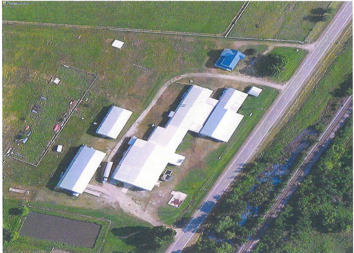
Designed to build fiberglass boats there are four separate buildings besides the office building: assembly- 50x150x14, lamination in 3 parts - 225x50x14, 100x100x16 and 50x100x18, R & D 50x100x14 and warehouse - 60x150x18. There are 3 spray booths and foam room. The facility is serviced by a 2 inch gas line w/5 PSI, 480 volt 3-phase electric.
